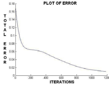
Fig. 7. The Neural Network adequately classifies the 15 training patterns after 1,184 iterations with a total-error below 0.02
